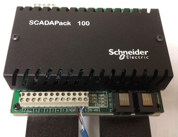
Figure 21 - SCADAPack 100 With Attached CAT5E Cable
